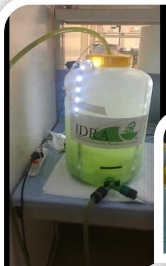
20 L Photobioreactor Prototype
